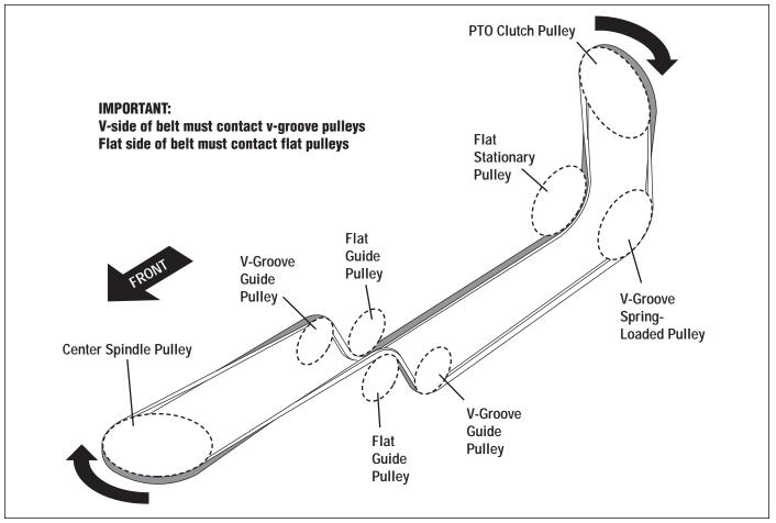
Figure 49. PTO Belt Routing
